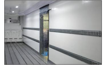
Side doors can be configured on one or both sides of the trailer based on your specific needs.
