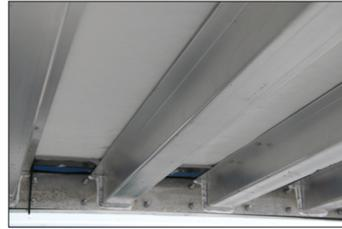
The use of a common end plate reduces the weight of the trailer by eliminating one crossmember yet adding additional strength.
