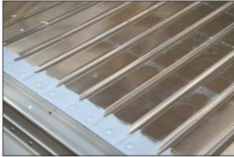
Corrugated roof sheet reduces stress between the foam bond and aluminum skin during thermal expansion.
