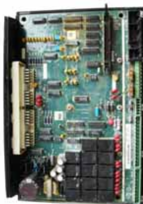
Badly corroded printed circuit board
