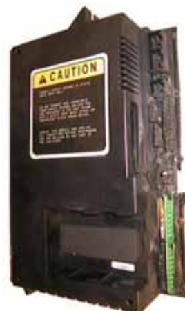
Badly burned printed circuit board
