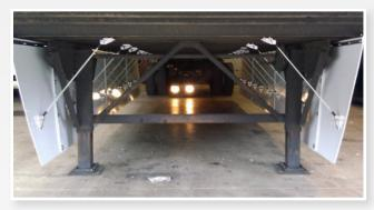
Flexible braces and basic AeroFlex components are simple, effective and proven through years of successful fleet use.
