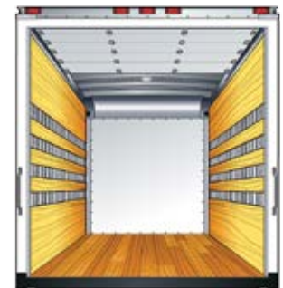
Universal: Plywood lining up to 24" from floor and down 24" from ceiling with 3 rows of slats evenly spaced in center.
