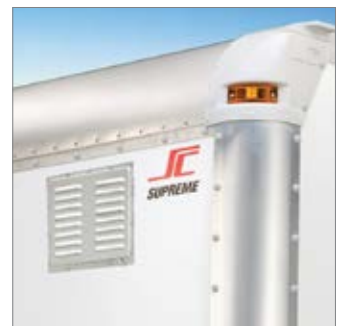
Wall vents for fresh air circulation inside your truck.
