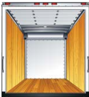
Standard: 3/8" plywood lining full-height side walls.
