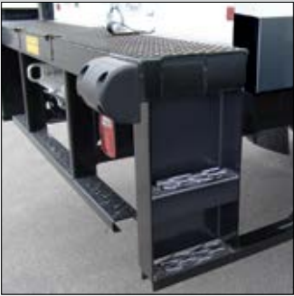
Rear floor extension with dual rear side steps, pooched ICC bumper and dock bumpers.
