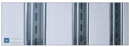
Recycled, high impact resistant white HDPE panels between slotted logistic posts snap in for ease of repair. The white panels also brighten the trailer interior for better visibility.
