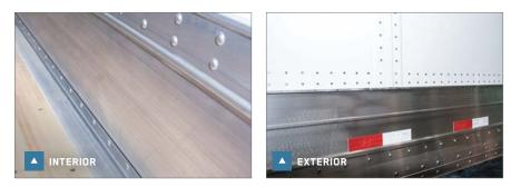
The bottom rail/integral scuff band has a centrally located external rib for increased stiffness and scrape resistance. The 16" integral scuff offers a smooth surface to prevent freight snagging and ribbed protection against pallet damage to the sidewall rivets as well as adding strength to the trailer body.
