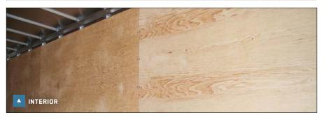
Plywood is installed horizontally over the side posts full length of the trailer and over the front wall.
