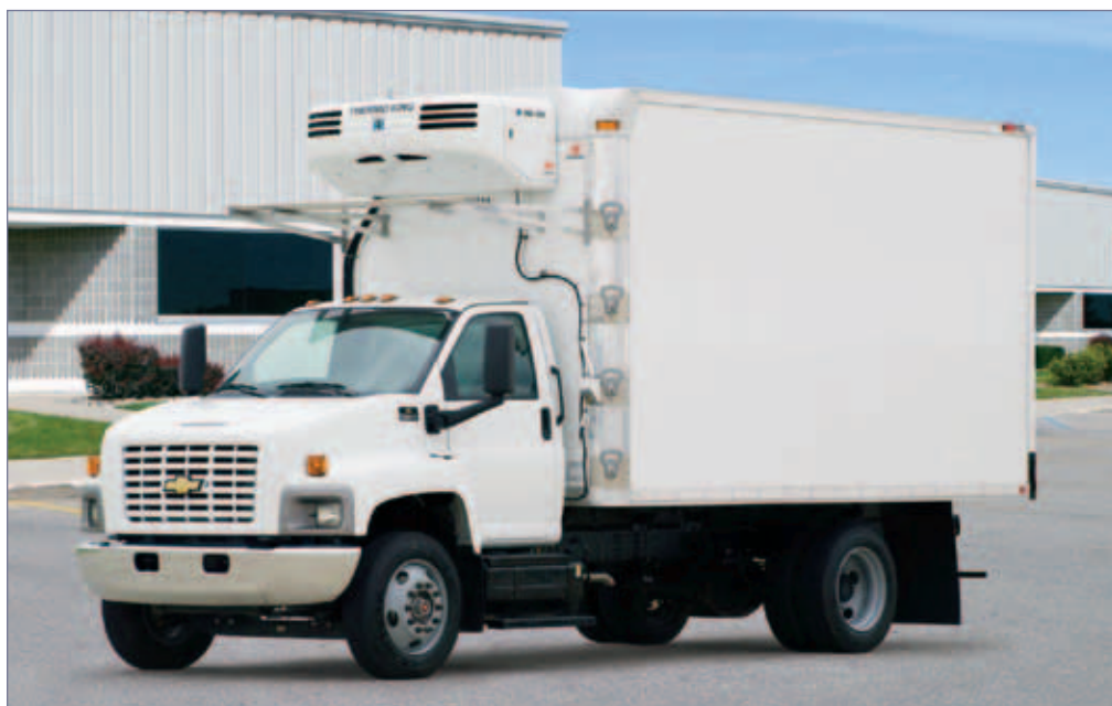
14' Aluminum Kold King with self-contained mechanical refrigeration unit
