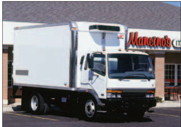
14' Aluminum Kold King with stainless steel vertical corners
