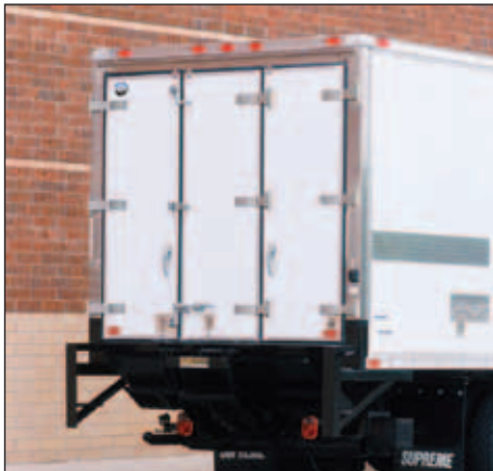
Tuck away lift gate allows dock loading.
