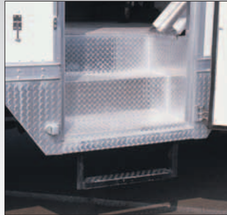
Insulated aluminum recessed stepwell with stirrups step provides easy curbside access to cargo.
