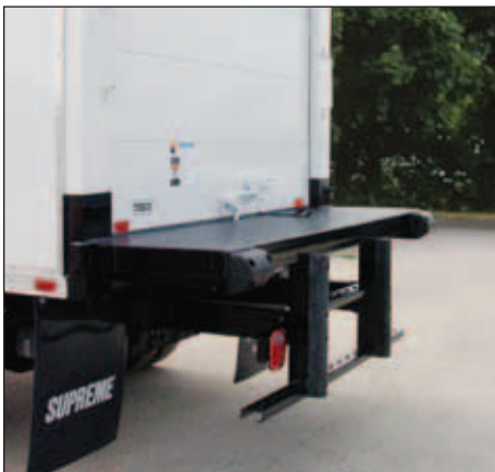
24" floor extension with ICC bumper provides an efficient loading and unloading platform.
