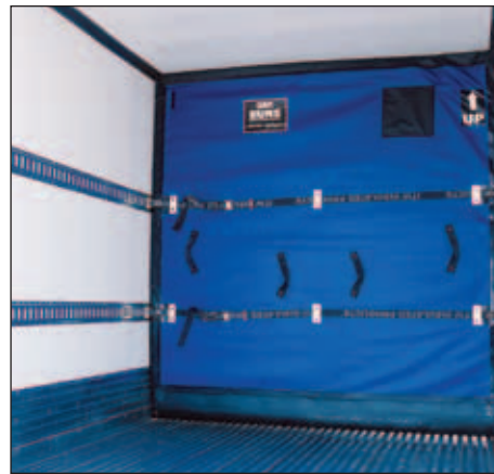
Scuff plate, E-track and Skinny Buns™ portable bulkhead for dual temp capabilities.
