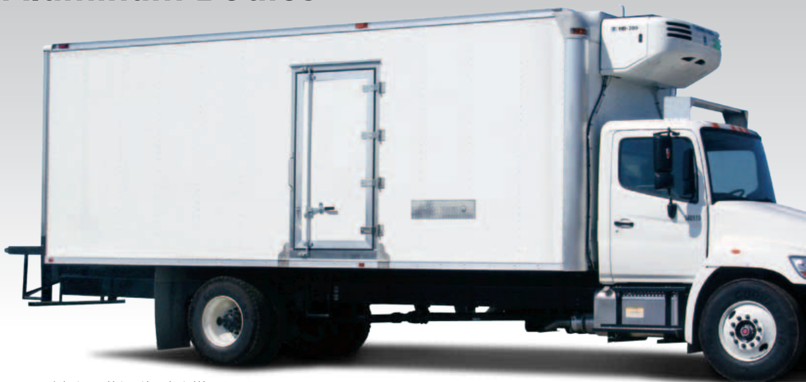
24' Aluminum Kold King with mechanical blower
