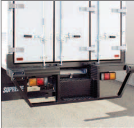
Chicago style step bumper and 3-panel door with ramp provides two ways to access the body.
