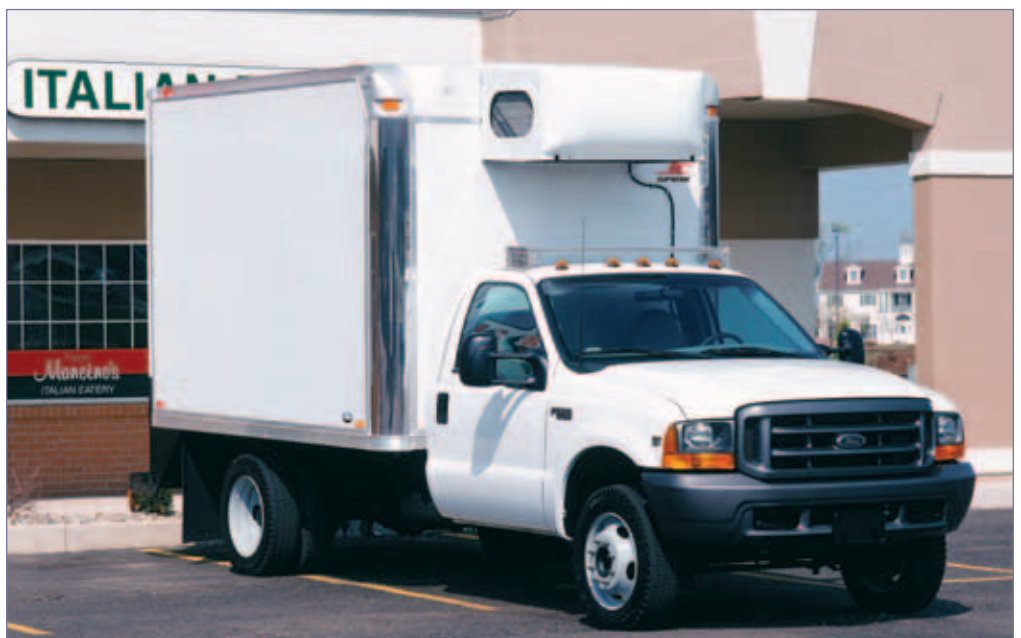
12' Fiberglass Kold King with front nose mount cold plate condenser
