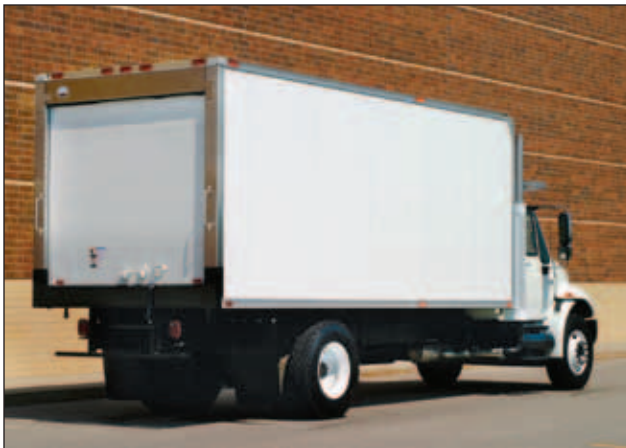
20' Aluminum Kold King heavy duty stainless rear frame and roll-up door.
