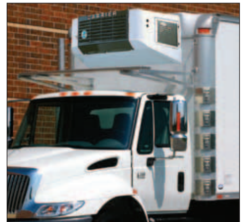
Reefer service platform, fold down reefer access steps makes servicing the reefer safe and easy.
