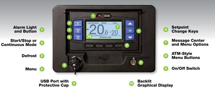
A large dashboard-style display shows all key operating information, providing an at-a-glance visual indicator of both unit operation and conditions inside the trailer.
