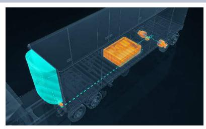
The zero-emission refrigeration system utilizes regenerative energy captured by the leading-edge energy recovery and storage system and stores it in a battery under the trailer (orange) for use by the Vector refrigeration unit mounted on the front of the trailer.
