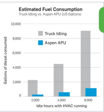
Truck idling fuel consumption –  $1.15 \text{ gph}^1$ Diesel APU fuel consumption –  $0.15 \text{ gph}^2$  At \$4 a gallon for diesel, use of an APU can generate savings of \$16,000 in reduced fuel usage after only 4,000 hours of use.
